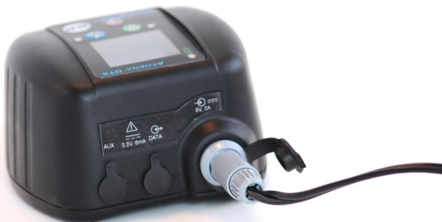
**Figure 15. WVSM™ Battery Recharging**
